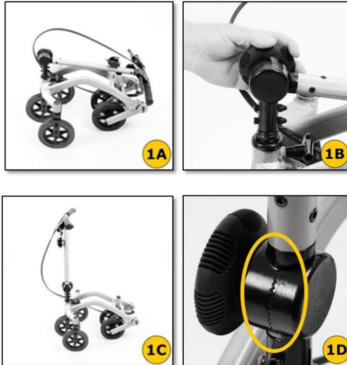
**⚠ WARNING:** Failure to ensure the teeth of folding mechanism are locked and secure may result in serious injury (Figure 1D).
