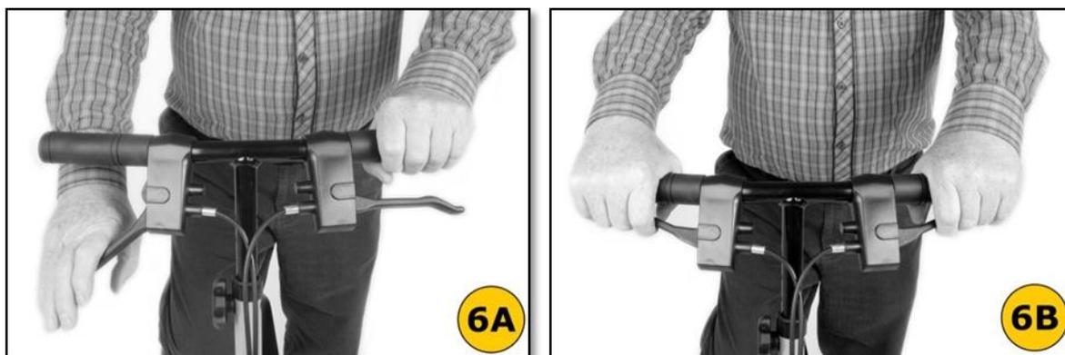
**⚠ WARNING:** Always engage the parking brake before mounting or dismounting the StrideOn. The StrideOn brakes are there to help slow the unit down, they are not intended to completely stop the unit
